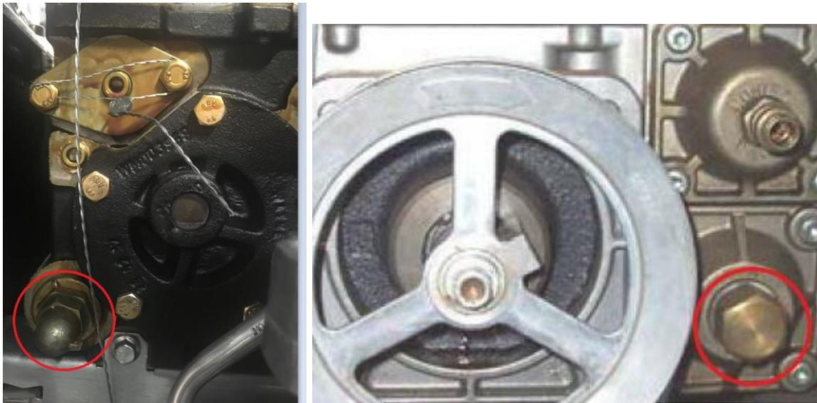
The bypass pressure setting in the factory full fill the requirements for the wet test of the dispensers. The conditions on site will be very different from the conditions on our factory test bay. For that reason, this has to be adjusted at installation.
