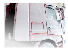
The automatic application of the chemical pre-wash saves time and controls consumption by service; its foamy texture ensures greater efficiency in the chemical through a longer reaction time on the vehicle surface. This optional extra includes stainless steel pipes and foamers for air mixing, a 100 L pre-mix tank and a high-pressure pump working at 100 bar and 28 L/min.
