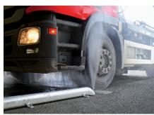
Drive-through underchassis wash with high-pressure, working at 70 bar and 126 L/min. With entry photocells for an automatic operation and 10 high-impact nozzles, it is installed at the start of the bay. It can work with the same high-pressure pump rack that feeds the rollover by means of a solenoid valve.
