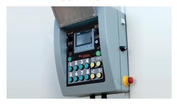
The external control panel with a colour touch-screen facilitates **user-friendly navigation** on the machine menu. It is equipped with push buttons for machine and brush manual movement, selection of up to 15 programs, and the possibility of on-line connection for remote control. A flexible configuration allows the user to set programs by wash pass, optimising speeds on each individual pass.
