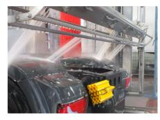
Especially developed for the touchless wash of the vehicle front and upper areas or to enhance cleaning results with demanding vehicle fleets. It works with 16 zero-angle nozzles at 70 bar and 126 L/min. and with an oscillating motor and a spinning motor for software-controlled 180° motion.
