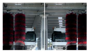
The self-driven vertical brushes perform an overlapping scrub on the vehicle front and rear. Brush positions are controlled by means of an encoder and the brushes of high-density polyethylene work with three pressure levels for the different vehicle shapes. Patented front tilting system – for improved cleaning results on the windscreen – is optional.
