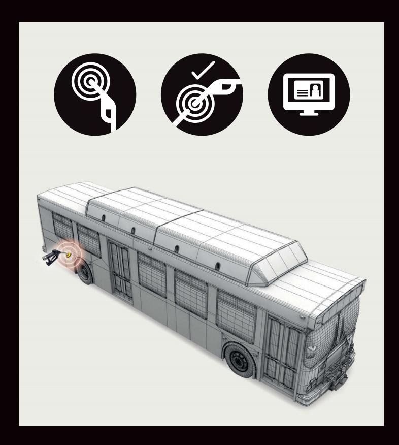
SmartFuel is Tokheim's automatic vehicle identification solution. It is an automated refuelling system that incorporates fuel authorisation based on vehicle identification. It has been designed for companies operating their own fleet of commercial vehicles to help reduce fraud and overcome many of the limitations inherent in traditional data input technology.
